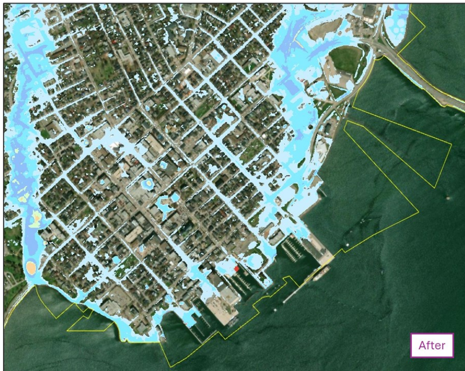
Figure 32. Comparison of the pluvial flood maps before and after applying the new boundary mask.
